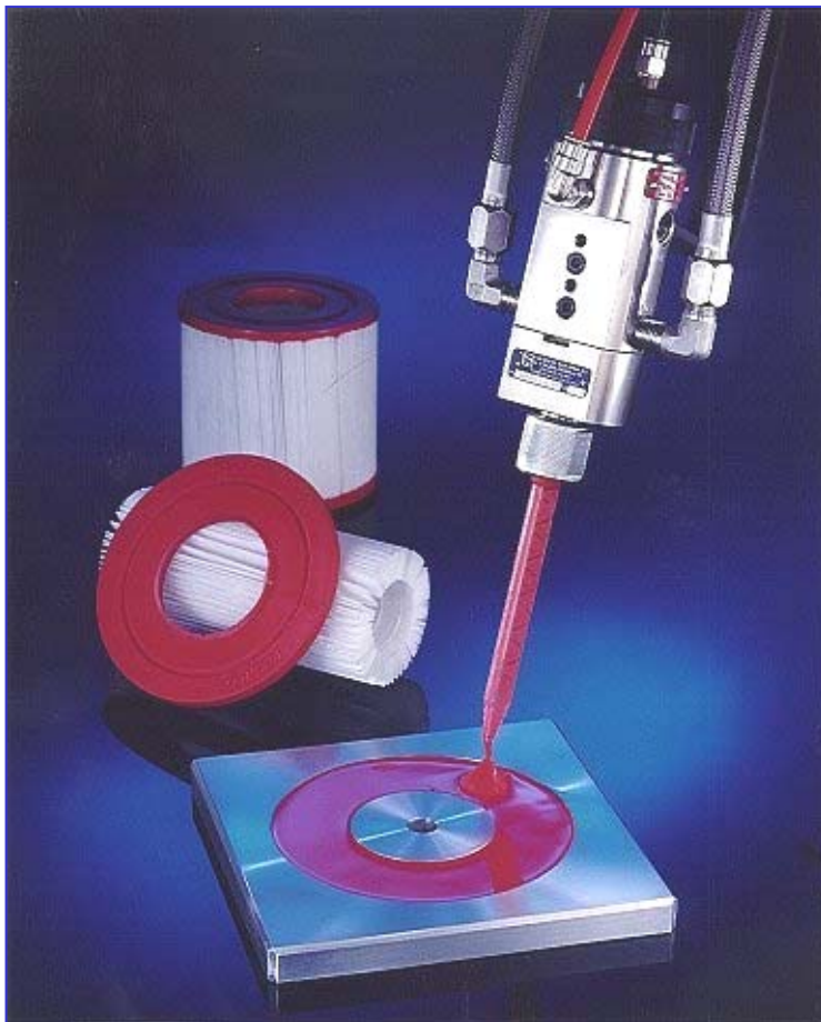
2-component polyurethane is applied into the end cap mold prior to inserting the filter element
